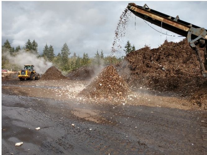
Figure 6: Mixed FSP and feedstock materials ground and coming off the conveyor prior to placement in quadrant for active composting at Olympic Organics.
